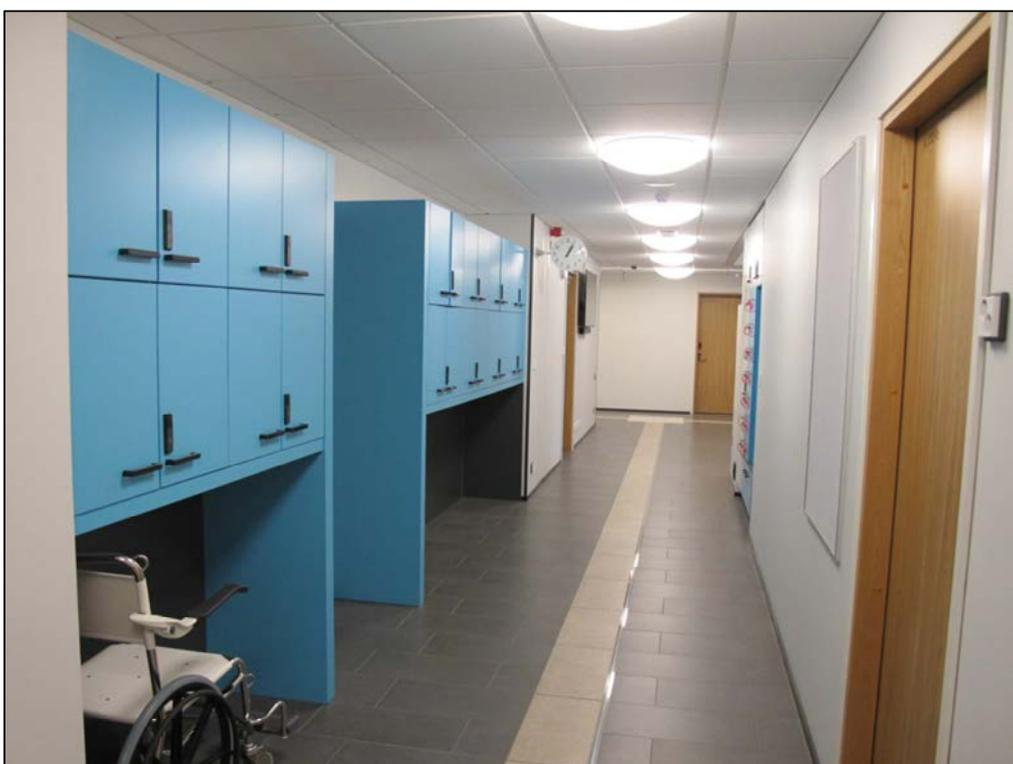
This is a hallway. Wheelchairs can be stored at the sides of the hallway. The flooring uses clear and distinct coloring and materials, which can help serve as guides for visually impaired children walking with the aid of white canes. At crossroads, it is easy to tell when a path is for a different facility, and it is easy to change directions if necessary.
