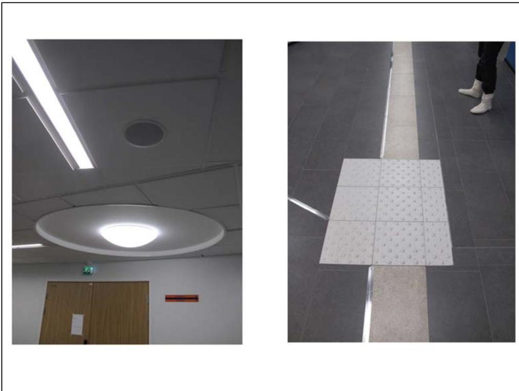
Speakers are installed in the ceiling. These speaker send signals to students pertaining to where they are currently located. For example, if you were to hear the sound of tableware from the speakers, it would mean that you are close to the kitchen. If you heard balls bouncing, you would know you are near the gymnasium. This is the pattern used on the floor.
