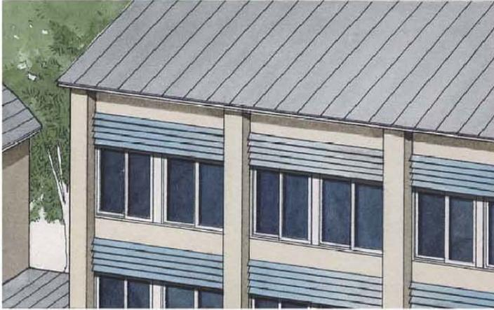
Solar cell modules are installed outside the windows\* or any openings of the school building, serving as window shades or blinds. They are similar to the modules fixed on window roofs, in that the panel dimensions depend on the manufacturer, the modules are usually custom-fabricated, and the modules are used for shading the sun; however, these modules differ in terms of where they are installed.
