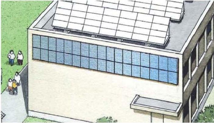
Solar cell modules are installed on the wall\* of the school building. Standard types of solar cell modules can be used. Modules with see-through perforated solar cells or those allowing light transmission between cells can be used in windows.
