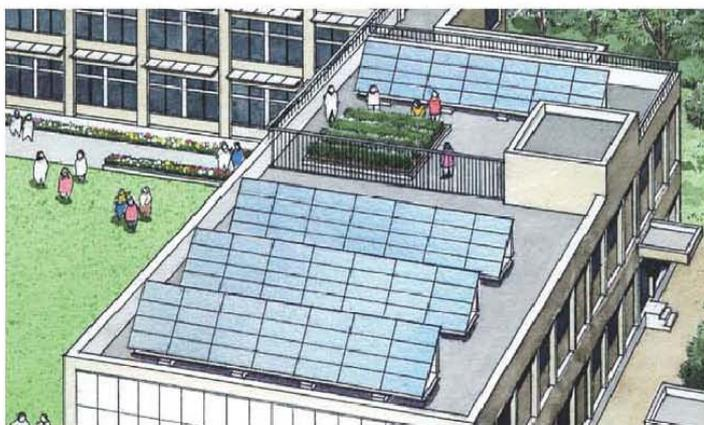
Solar cell modules are installed on a flat roof of the school building. Mounting frames are necessary for tilting the solar cell panels to ensure maximum power generation efficiency. A concrete foundation may be needed for fixing the mounting frames.
