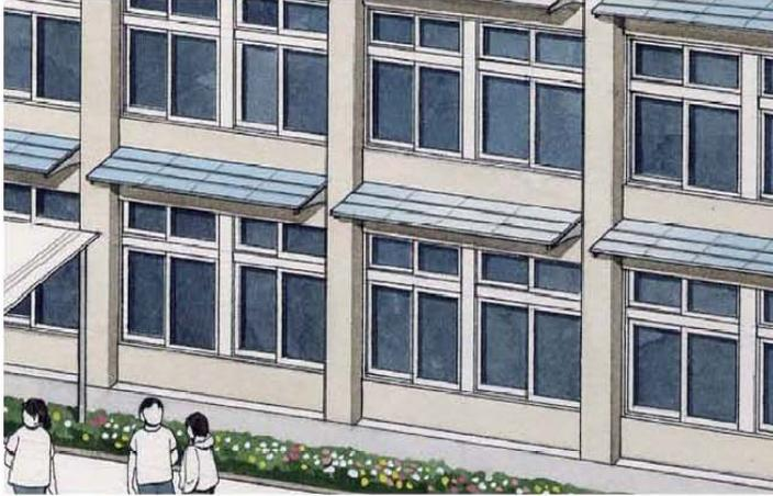
Solar cell modules are installed above windows on mounting frames\*. The modules serve as window roofs and can be used as sunshades. The panel dimensions depend on the manufacturer, and modules are usually custom-fabricated.
