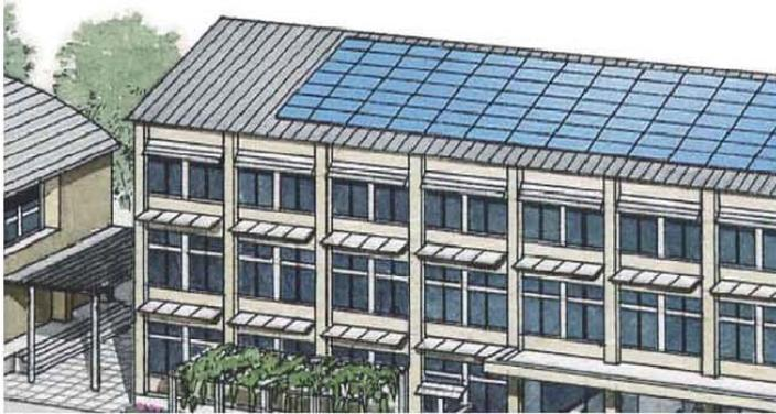
Solar cell modules are installed on the sloped roof of a school building. Because the modules are fixed almost flat on the roof surface, a roof facing an appropriate direction should be chosen. Care may be needed to determine the module design in terms of color, quality of material, shape, etc., because modules on a pitched roof\* are conspicuous.
